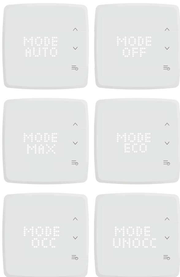
Figure 2-5 Indications in the controller display 3
