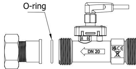
9. It is important to verify the maximum torque applied to the hexagon of the device because the plastic body of the flow meter can be damaged. In the following table is reported the recommended torque, referred to as the nominal diameter (DN).
