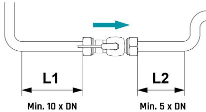
5. As shown in the images below, the flow meter can be mounted in all positions except for the case in which system filling problems may arise (See example at point 6).
