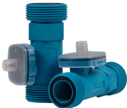
*Flow-meter is a direct type of flow-measuring device with operating fundamentals based on the Von Karman principle. A piezo-elettric sensor detects the vortices, which are converted into an electrical frequency signal.*
