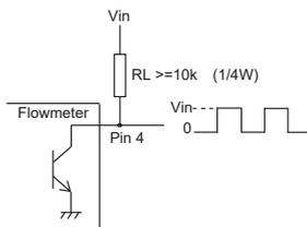
**Note:** the frequency output is a square wave with 50% duty oscillating between Vin (positive power supply) and ground. The frequency is available on Pin 4, an external resistor must be mounted between Pins 4 and 1 ( $RL \geq 10 \text{ k}\Omega$  1/4 W).
