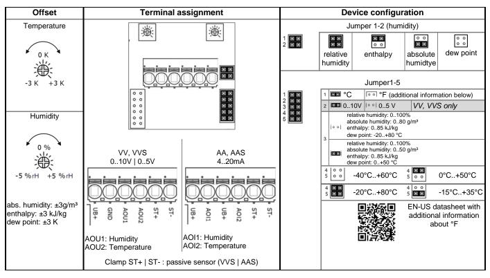
The adjustment of the measuring ranges is made by changing the jumpers in a de-energized state. The output value of the new measuring range is available after 2 seconds. *fig. (Measuring range and offset adjustment, default settings: -20 °C.+80 °C | 0 K)*
