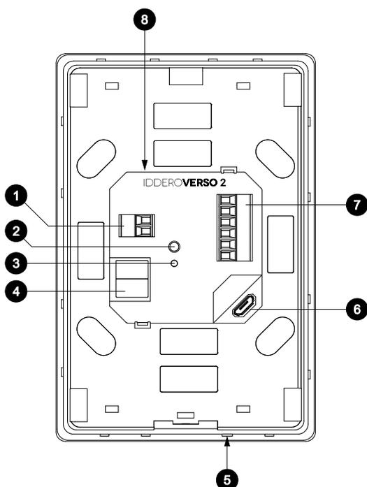
1. Power supply connector (12-30 VDC)
