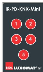
In the DX variant, a mini remote control is available for the end customer, which can be programmed according to the end customer’s wishes and can also be used for remote control of other actuators present in the system. Since the information is stored in the detector and the remote control only sends one infrared command per button, a different programming of the remote control can be stored in each detector.
