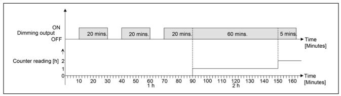
The totalled operating hours are added in a 2-byte counter and stored permanently in the device. The current counter status can be transmitted cyclically to the bus by the "value operating hours counter" communication object or when there is a change in an interval value.
