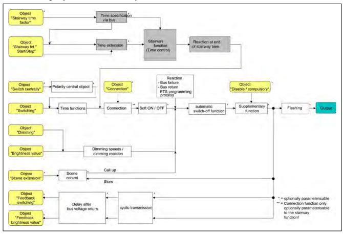
Time-independent continuous light switching can also be implemented in combination with a disabling function because the disabling function has a higher priority and overrides the switching state of the staircase function.
