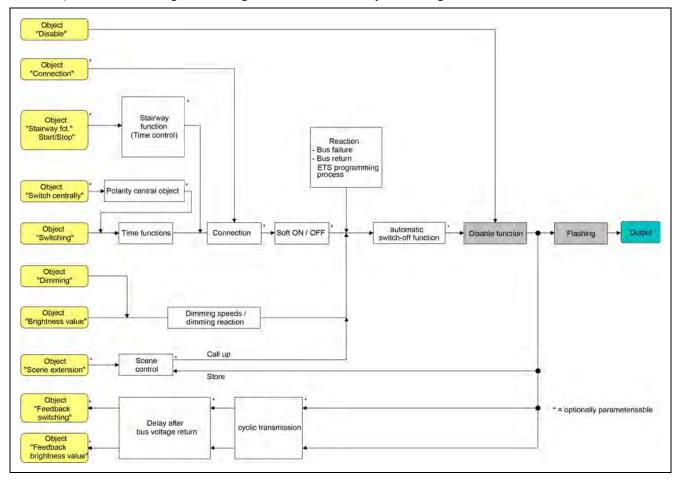
On the parameter page "Kx - Supplementary functions", set the parameter "Selection of supplementary function" to "Disabling function".
