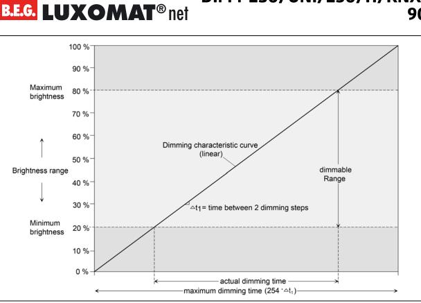
In some practical applications, a linear dimming characteristic is not optimal. Hence, the actuator in the ETS alternatively permits a user-defined adjustment of the dimming progress. In this way, for example, brightness changes can be adjusted to the brightness sensitivity of the human eye when dimming by subdividing the brightness range in up to three sections with different dimming increment times.
