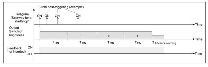
With this function, the lighting time in a staircase can be extended (e.g. by a person after shopping) by a defined length without having to retrigger the lighting every time the lighting shuts off automatically.
