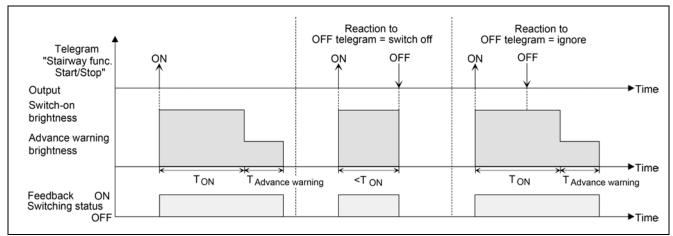
In addition, the switch-off can be influenced by the soft functions of the actuator. Taking into account any soft ON and soft OFF function, this gives rise to a modified switch-off behaviour of the staircase function.
