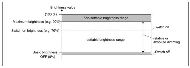
Definition of the lower brightness limit with minimum brightness:
