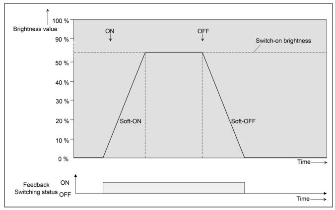
The dimming speeds can be configured separately in the ETS for the soft ON and soft OFF function. The relative dimming increment time between 2 of 255 dimming increments is configured directly.
