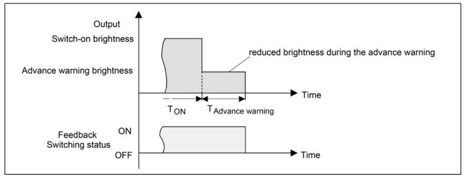
The pre-warning time influences the values of the feedback objects so that the switching state "OFF" and the value "0" is first tracked after the pre-warning time in the feedback objects has elapsed.
