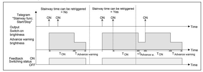
In addition, switching on can be influenced by the soft functions of the actuator. Taking into account any soft ON and soft OFF function, this gives rise to a modified switch-on behaviour of the staircase function.
