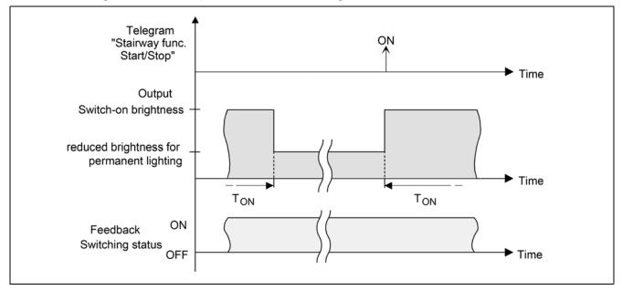
The continuous lighting remains permanently active after the staircase time has elapsed. Only when an ON telegram is received again via the object "Staircase function start/stop" does the actuator switch back to the switch-on brightness and start counting the staircase time again. The receipt of an OFF telegram via the object "staircase function start/stop" only switches the continuous lighting off if the parameter "Reaction to OFF-telegram" is configured to "switch off".
