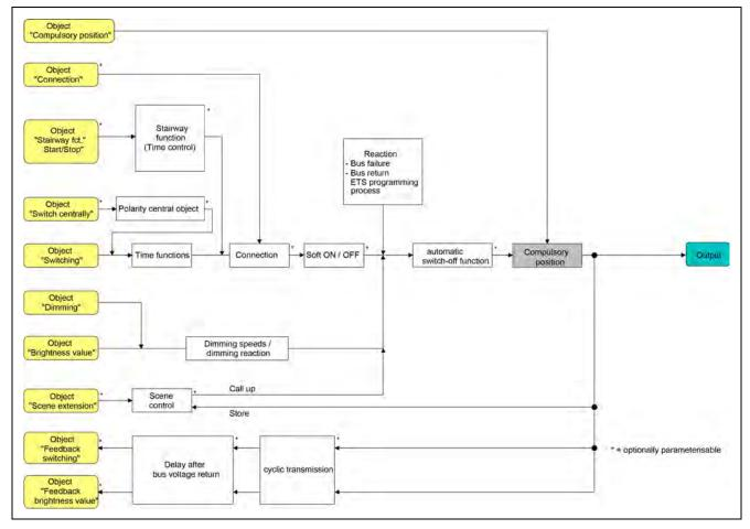
On the parameter page "Kx - Supplementary functions", set the parameter "Selection of supplementary function" to "Forced position".
