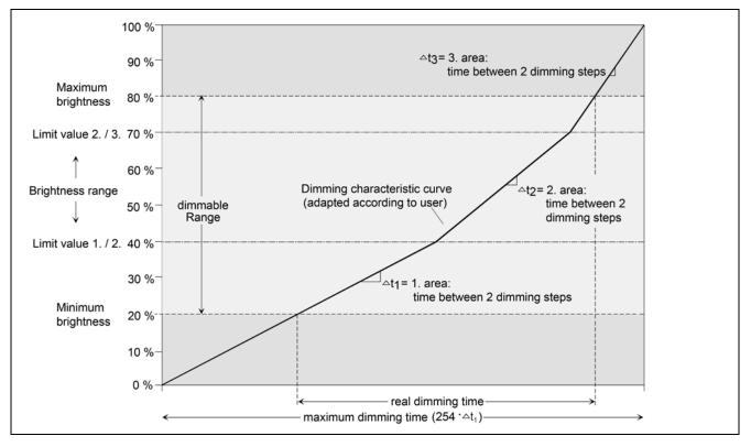
As an additional option, it is possible to set predefined dimming characteristics for incandescent lamps or for halogen lamps in the characteristic parameterization. In this way, the dimming progress can be optimised for the named lamp loads. In this case, the dimming actuator works with fixed implemented brightness sections and dimming increment times.
