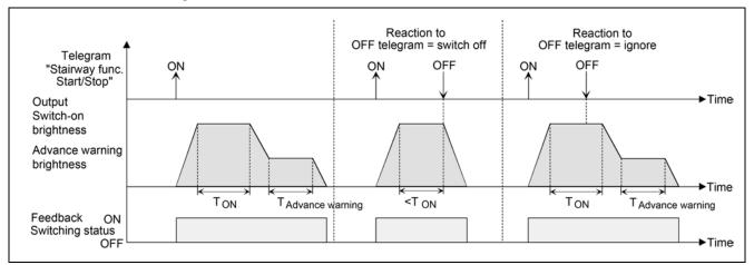
The parameter "Reaction to OFF-telegram" on the parameter page "Kx – Staircase function" (x = number of the dimming channel 1 ... 4), defines whether the staircase time ( $T_{ON}$ ) of the staircase function can be aborted prematurely.
