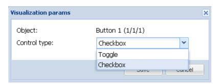
• *Control type* – type of the visual control element which will appear in Touch Visualization
