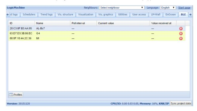
By clicking on specific device, you can map its functionality to KNX group addresses. For AWOX AromLight Color BLE lamp, you can map LED color object to KNX.
