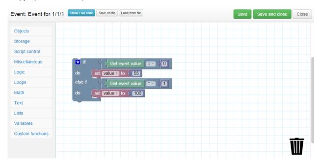
If the block is indicated with the blue label on the top left corner, you can define the structure of the block (e.g. If Else)
