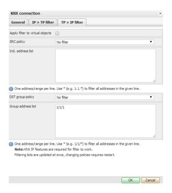
Apply filter to virtual objects – either to apply filter policy to objects added in Objects tab as virtual objects without attraction to bus
