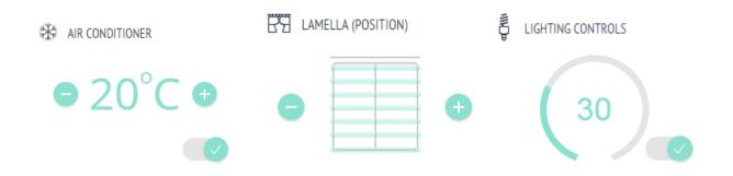
Now you can set a title for this widget and link KNX objects to widget's controls. After you've set up a widget click on the "Add this widget" button. Well done, the widget on the screen. Right-click on it to see/edit it's properties or delete the widget.
