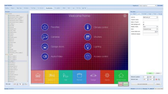
When all links are defined, press *Save and reload floor plan* button.
