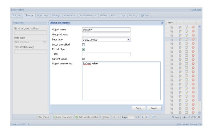
In System Configuration → Network →BACnet objects you can see marked objects on LogicMachine which are sent to BACnet network.
