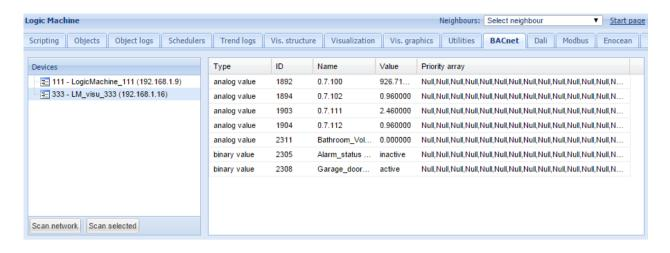
By clicking on *Scan Network* button you can see a list of BACnet server devices on the network. With *Scan Selected* you can rescan specific BACnet server for respective objects.
