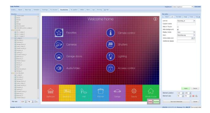
Objects can be added to the map by clicking on *Unlock current floor plan for editing* button. In this example we are creating first page of visualization which will link to other Floors with specific object control. Add link by clicking on Link tab, choosing specific icon, scale it and place in desired location.
