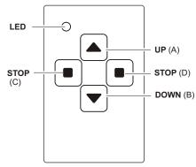
**RT30E5001-01** 868.30 MHz **RT30E4101-01** 433.92 MHz **RT30E6001-01** 916.50 MHz Function: 1x UP/STOP/DOWN 3-button operation
