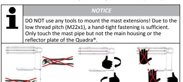
put the Quadra<sup>®</sup> with the mast extensions intoi the mast clamps, clos the clamps and fasten them with the screws – take care oft he orientation
