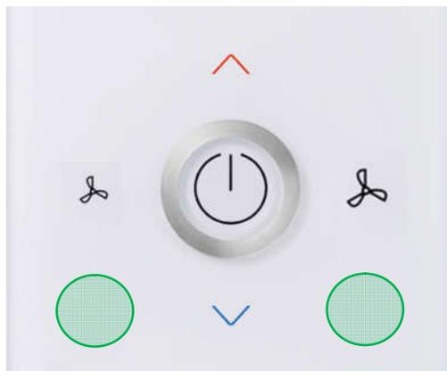
You can switch to cleaning mode with the two hidden buttons at the bottom left and bottom right. For this, the key combination must be pressed for at least 3s. The cleaning mode will last for 20s. The elapsed time is shown in the display. During this time, all buttons are locked.
