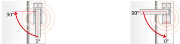
**VFG** Wireless sensor for changeover specification. As an alternative to the digital input, a radio changeover sensor can be learned-in.
