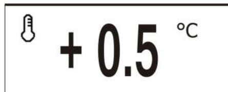
Picture 16 Display of set point adjustment
