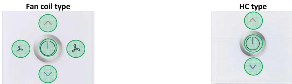
Single key actuation releases an action. A long keypress causes a cyclic value change in a 0,5s cycle.
