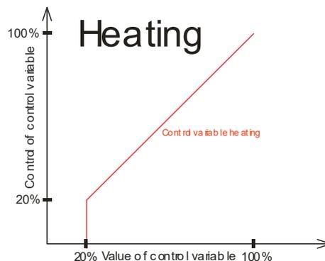
The control variable is only sent to the output, if the calculated value of the control variable is bigger than the minimal control variable
