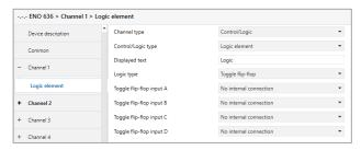
Each gate channel supports up to 4 separate toggle flip-flops:
