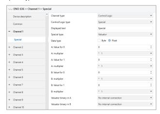
Each channel supports up to 4 valuators to output byte values, or up to 2 valuators to output 2-byte float values:
