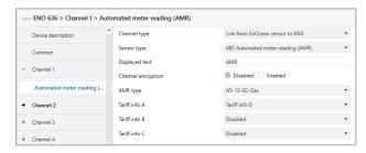
A maximum of three counter channels are supported for each channel. The counter channels that the EnOcean device transmits must be known and set in the parameter. Two communication objects are available for each counter channel, one for the current consumption and for the total consumption.
