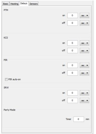
For all sensor types: An ON- and OFF-delay can be set from 0..99 sec or 0..99 minutes.
