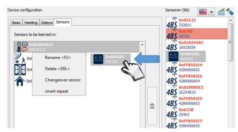
Sensors and devices, within range, are listed on the right side of airConfig. To learn in a specific sensor simply drag and drop the (activated) symbol into the sensors input tab of the STC-DO. The Sensor's (EEP) type must be known to be assigned correctly through activation of the sensor or switch. The sensor type is coded in the EEP, which is included in the sensor's LRN telegram.
