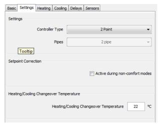
**Controller Type** can be set to 2-point control or proportional control (PI-loop) with PWM for thermal actuators.
