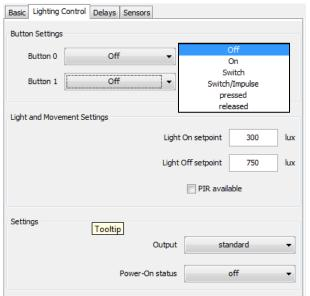
Any side of a rocker can be configured to work as ON, OFF, Switch (Toggle), Switch (Pulse), push button pressed or push button released.
