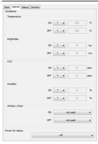
Custom programmable applications using 2-point control based on temperature, brightness, CO2, relative humidity or window status. Custom programs can be selected: "more – less – equals" can be selected in combination with a threshold to turn on or off the relay.
