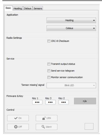
In the 1<sup>st</sup> tab "Basic", the "Application" must be selected using the drop down menu. Depending on the selected application airConfig will offer additional tabs to configure the device.
