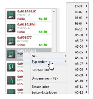
If the EEP of a particular sensor is already known, the EEP can be set manually by clicking right on the sensor's icon and selecting the EEP from the "change type" dialogue.
