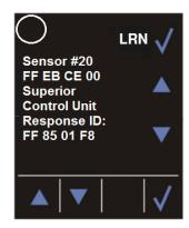
To finalise the teach-in process enter thanos' configuration menu by pressing the 2 buttons in opposite corners (i.e. lower left and upper right) for a few seconds. Browse to the menu to reach the teach-in of sensor #20 (Superior Control Unit):
