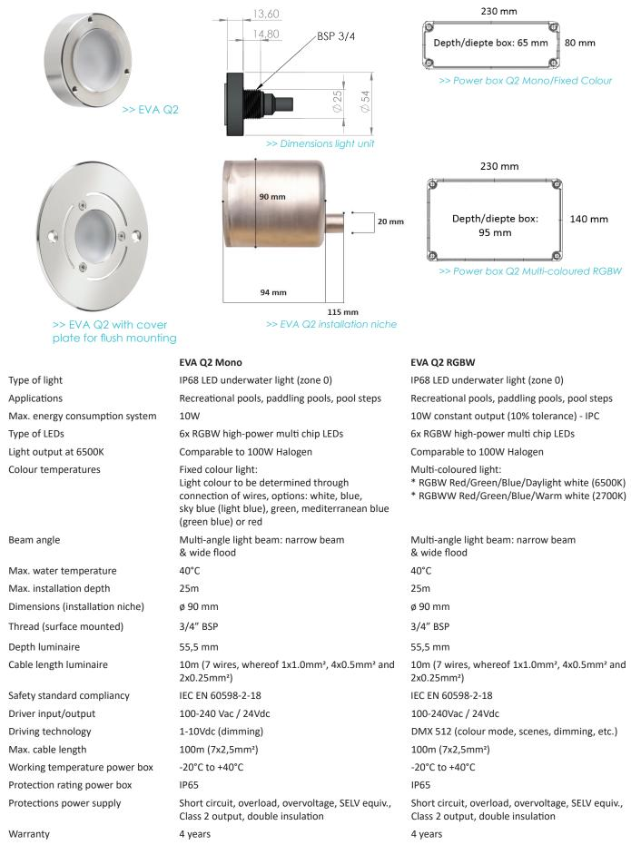
\* Important note! Always provide sufficient space around both luminaire and power box to allow for cooling
