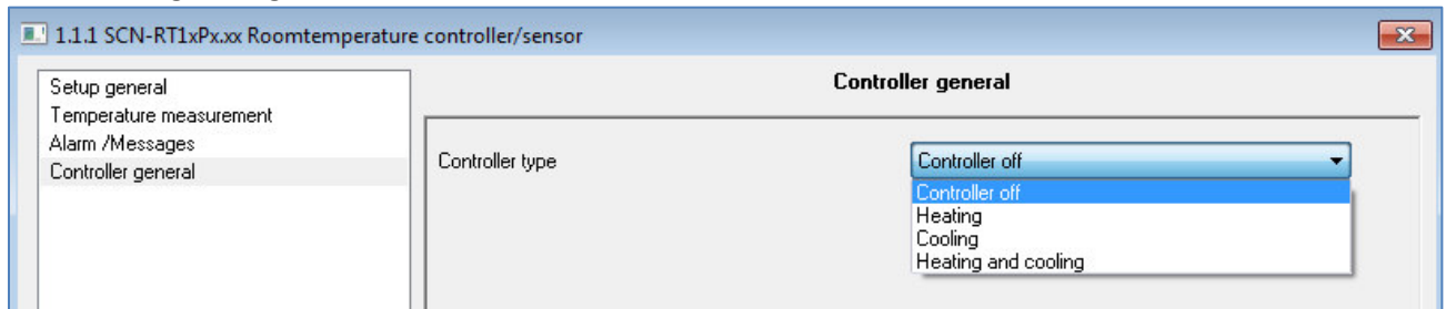
Figure 8: Setting controller type
