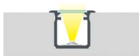
The end result of installation of recessed profile G with a BASIC cover
