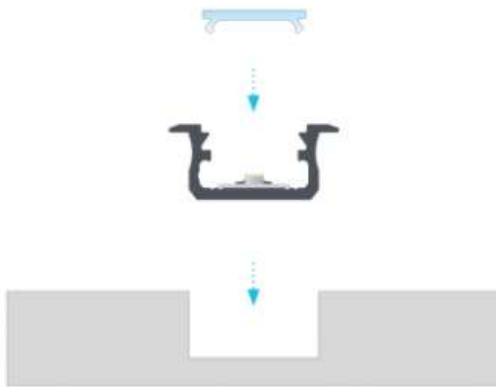
Installation instructions for recessed profile B with a BASIC cover
