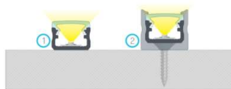
The result of installation of profile A with HIGH cover, (1) with double-sided tape (2) with a mounting clip for A
