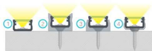
The result of installation of profile A with BASIC cover, (1) with double-sided tape, (2) with a mounting clip for A, (3) with A MINI mounting clip, (4) with metal mounting clip for A
