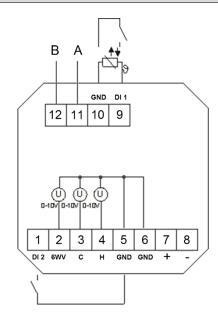
1 GND (6-way valve) 2 0..10 V (6-way valve)
