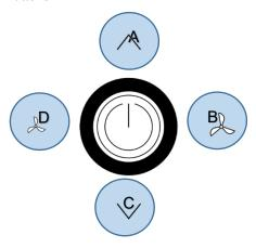
The configuration menu is activated by simultaneously pressing the buttons "up" (A), "left" (D) and "right" (B) for at least 3 seconds. Menu navigation on the touch-surface is performed by pressing the buttons "up" (A), "down" (C), "left" (D), "right" (B) or the power button. Choose the desired parameter and press "right" (B) to open up the submenu. If no entry is made for 8 minutes, the parameter menu is left automatically. To exit the menu select the header line and press "left" (D).
