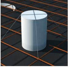
Fix the formwork unit to the reinforcement with tie wires.
