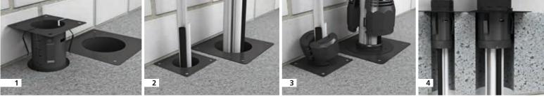
Installation takes place easily and quickly from the ceiling upper surface. The ceiling seal system can also be retrofitted around existing cables and conduits. Non-destructive later fitting of additional cables up to full population is possible at any time.
