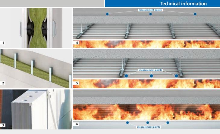
1 + 2 Construction of F90 metal stud walling acc. to DIN 4102 part 4.
