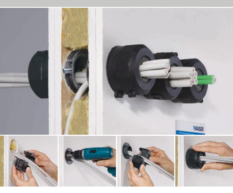
▲ Box sealing systems DS 90 / 74 mm and DS 90 / 120 mm consist of two parts which are pushed onto each other and locked. Push the sealing cylinder, which uses AFS-technology to close the wall, into a Ø 74 mm or Ø 120 mm cut opening and fix it, exactly like a KAI-SER cavity wall box. Then place the sealing element round the cables, push it on to the sealing cylinder and close it by turning it to the right until you hear an audible click. This guarantees secure room separation.
