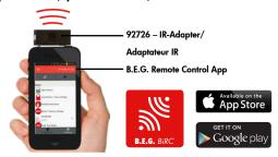
The device can be set up using the IR adapter and B.E.G. remote control app. No settings can be made on the device itself. The "B.E.G. LUXOMAT® Remote Control" smartphone app is available free in the Apple App Store and the Google Play Store.
