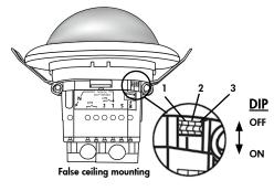
DIP 1 Fully automatic/semi automatic mode
