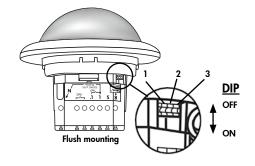
DIP 1 Fully automatic/semi automatic mode
