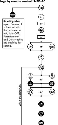
Unlocking device - Activation of the programming mode
