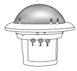
LED 1 green LED 2 white LED 3 red Potentiometer 1 Lux Channel 1 Potentiometer 2 Time Channel 1 Potentiometer 3 Time Channel 2
