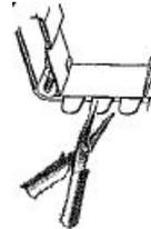
The interface can control up to 2 x 8-channel Wiring centres. If you have more than 8 zones, you can connect two modules together on the bus terminal (no. 3). In this case, it is necessary to put one of the modules in slave mode by turning the first dip switch to ON:
